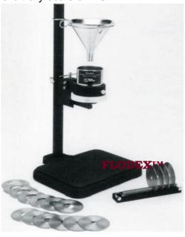
The tester has demonstrated its applicability and usefulness to determine a quantitative measure for non-free-flowing metal powders and premixes. It complements the Hall Flowmeter to characterize flow quantitatively and scientifically for the practicing engineer.
